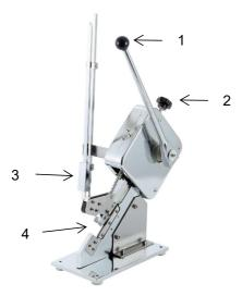
1.Handle 2.Locking screw 3. Pressing block 4.Buckle area
